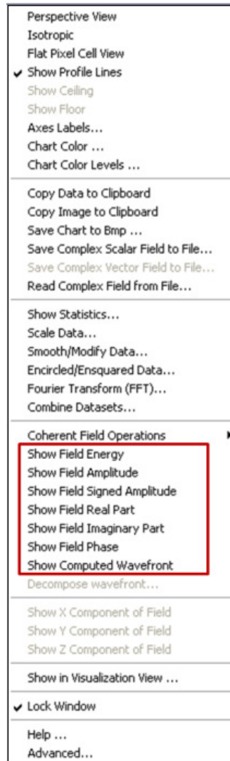
Figure 9. The Scalar Field Analysis menu is displayed when right-clicking the plot. Red box shows available plots.
